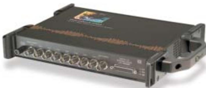
WaveBook/516A includes a parallel port for connecting to the WaveBook/516E
